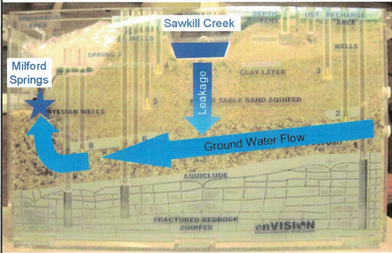
This table-top model simulates the flow of ground water through the sand and gravel aquifer to the Milford Springs. Dye is used to trace the leakage of water from Sawkill Creek into the aquifer and the flow to the springs. Dye also shows how a leaking heating oil tank and a malfunctioning septic system seepage bed can contaminate ground water. Arrows have been added to this photo to indicate the paths of flow when the model is operated using an aquarium pump.
